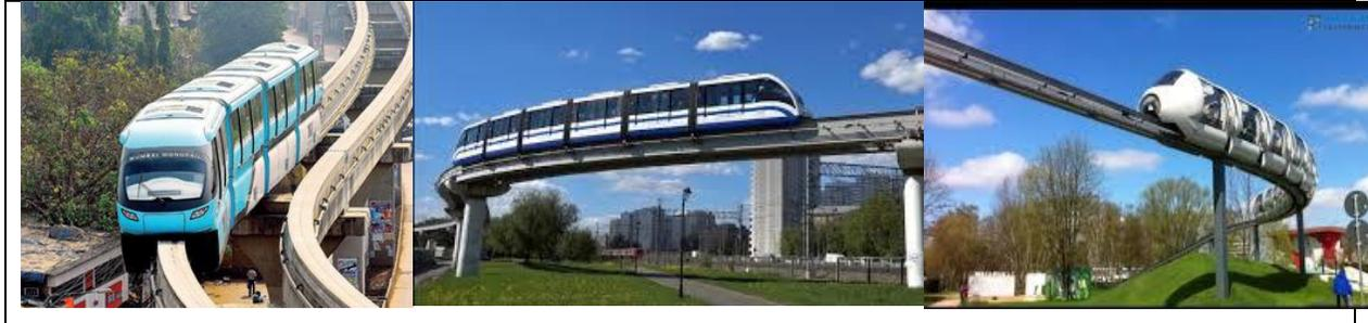
FIGURE 1. STRADDLE TYPE OF MR STRUCTURE
