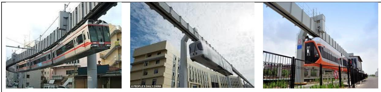
FIGURE 3. SUSPENDED TYPE OF MR STRUCTURE
